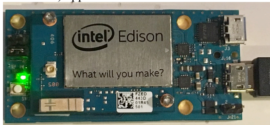
Figure 1: The Intel Edison with a Mini Breakout Board from Adafruit.com.
